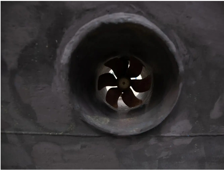
BOW THRUSTER, WELDED IN STEEL
